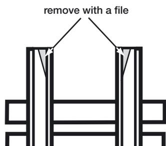
filing the inside ball of the rail at a slight angle for about 3/16" (4mm) (see illustration above).
